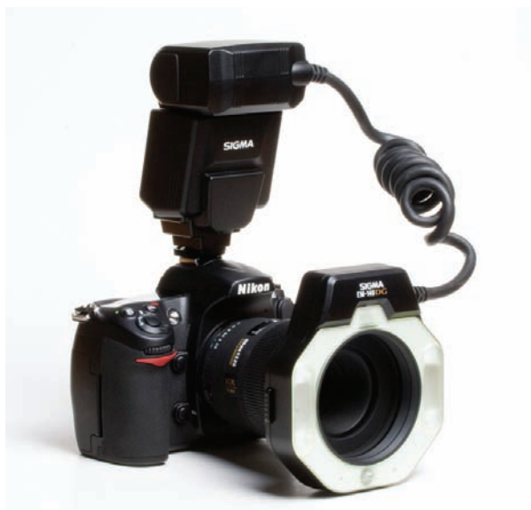
FIGURE 1 Nikon DSLR with a Twin Point Flash & Ring Flash configuration (photograph courtesy of Photomed).
